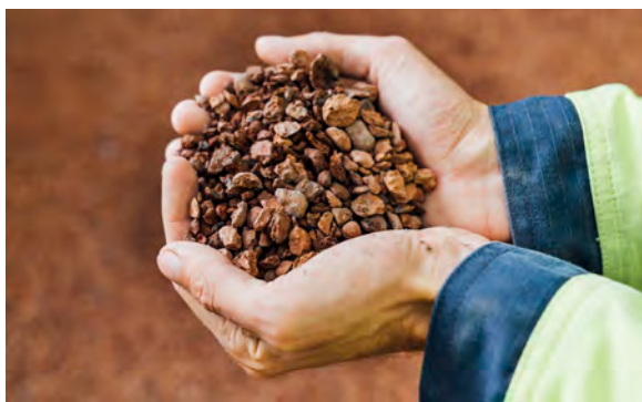
Calcined clay a low carbon material was used in the production of Futurecem.
