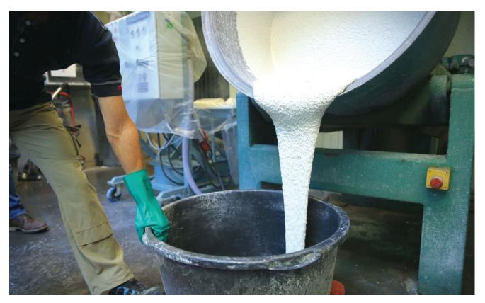
Mixed at a 1:10 ratio by weight, water and Aalborg Excel yield a self-consolidating mortar that exhibits flow characteristics of 300 ± 20 mm for 45 minutes or longer, per ASTM C 230, Standard Specification for Flow Table for Use in Tests of Hydraulic Cement guidelines. The white color is ideal as a base for architectural ultra-high performance concrete, which can be designed with coloring agents and conventional or specialty fine or coarse aggregate.
