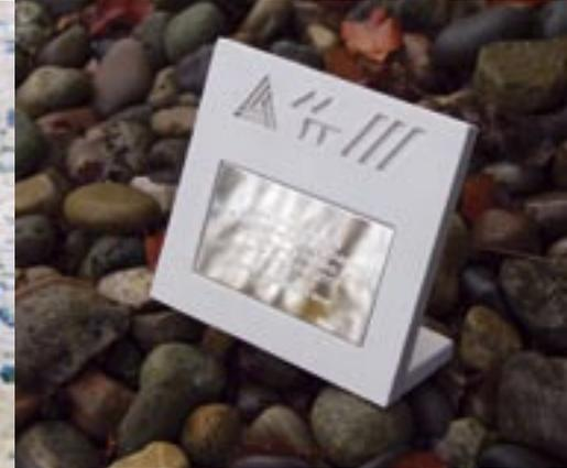
*To achieve the desired surface expression, care must be taken during casting to ensure that the formwork, not the casting, defines the texture of the finished surface.*
