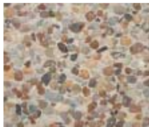
Exposed surface with fine pebble gravel 16/32.
