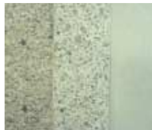
Exposed, polished and acid-etched surface with Blauschwartz (7/15 (German aggregate).
