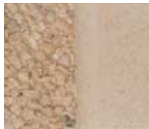
Exposed and acid-etched surface with Lahn quartz 5/8 (German aggregate).
