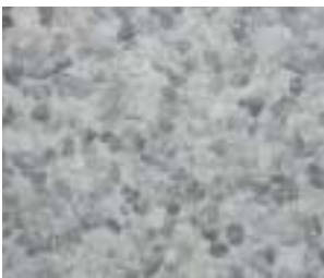
Exposed surface with Hardeberga granite.
