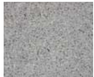
Acid-etched surface with Bayergrün 10/20 (German aggregate).
