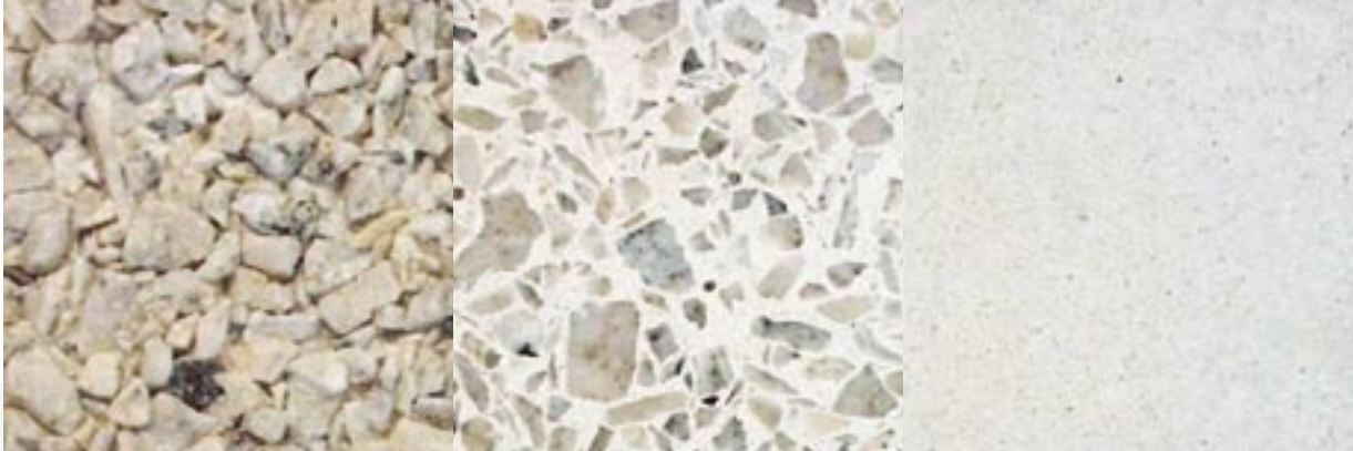
Three different surface expressions from the same concrete composition, left to right: exposed aggregates, polished and acid-etched.
