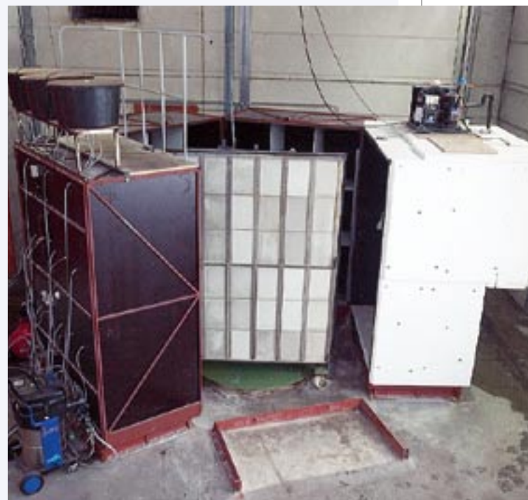
Instrument developed at RDC for accelerated aesthetic ageing. Thirty six concrete samples of the size used in the colour measurement instrument are exposed to frost, a light water spray, UV lighting and heating, and a light dust spray. Twenty four cycles are equivalent to approximately 1 year of outdoor exposure.
