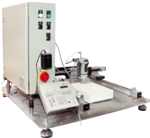
Instrument specifically developed at RDC for the aesthetic evaluation of concrete. The surface colour of 25×35×7 cm concrete tiles is measured at 96 points and the mean used for evaluation.
